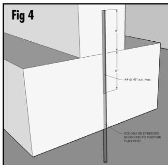
There are several methods that foundation contractors can use to reduce the likelihood of a problem. First, keep the height of the backfill to no more than 4' except at the corners or offsets until the deck is in place. Four feet of unbalanced backfill will usually not exert sufficient pressure to damage the wall.
