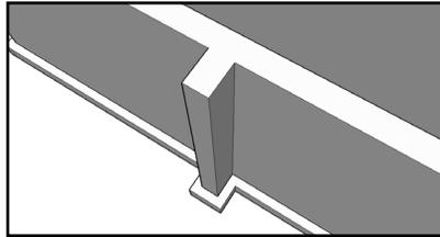
The type and consistency of soils greatly impacts the design lateral load on foundations. Consequently, the backfill condition should be considered during the design of the foundation wall. If the original soil excavated from the over dig is to be used, the wall must be designed for the resulting soil pressures. The pressure on a foundation can be reduced if well-draining soils or granular fills replace the excavated native soils.
