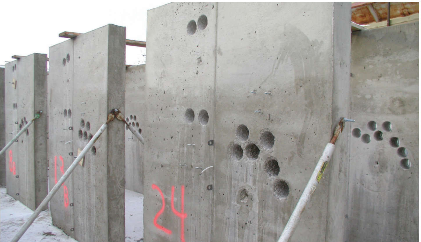
Fig. 3: The remaining wall segments following core sampling to compare to the cylinders taken during placement.
