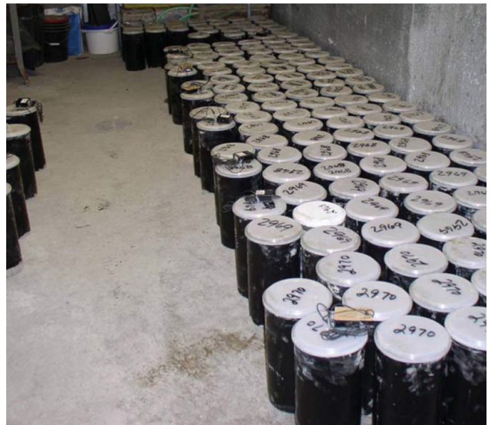
Fig. 1: The refrigerated test chamber at Master Builder’s laboratory in Cleveland, OH with all cylinders from Phase I ready for testing. Note the maturity meters in cylinder 1 of each set.
