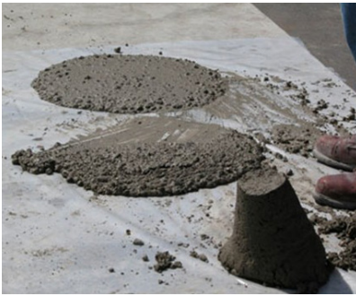
Fig. 6: Regular slump shown in a cone and SCC concrete shown in a puddle or flow.
