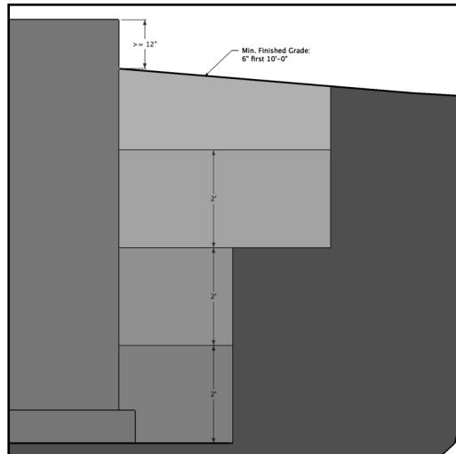
**Fig 7: Backfill in tamped lifts and finish with proper slope**
